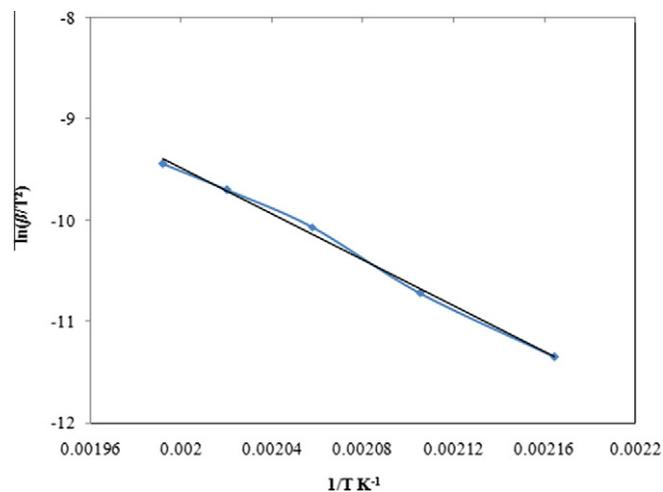
Fig. 4. Kissinger's approach to determine kinetic parameters for complex  $\text{C}^3$ .
