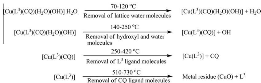
**Scheme 3.** Thermal fragmentation of complex  $[\text{Cu(L}^3\text{)(CQ)(H}_2\text{O)(OH)}] \cdot \text{H}_2\text{O}$ .
