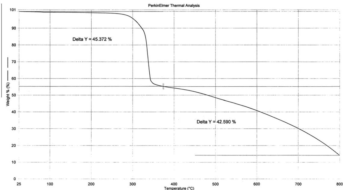
Fig. 1. TG curve of the complex  $[Cu(L^3)(CQ)(H_2O)OH] \cdot H_2O$ .
