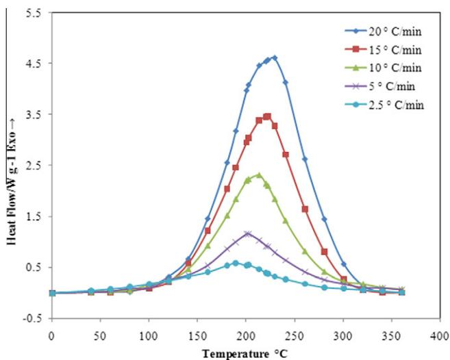
Fig. 3. Dynamic scan DSC curve of complex  $\text{C}^3$ .
