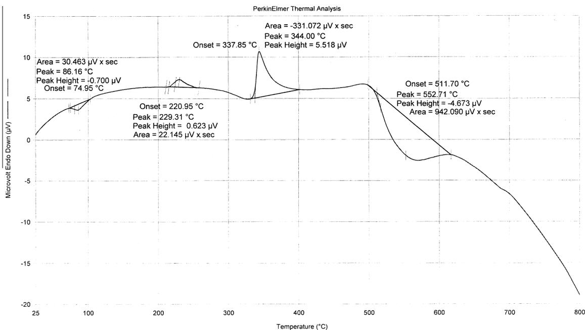
Fig. 2. DTG curve of the complex  $[\text{Cu}(\text{L}^3)(\text{CQ})(\text{H}_2\text{O})\text{OH}] \cdot \text{H}_2\text{O}$ .
