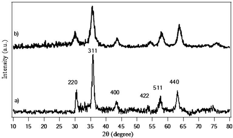
**Fig. 2** The XRD pattern of Fe<sub>3</sub>O<sub>4</sub> magnetic nanoparticles (a) and Fe<sub>3</sub>O<sub>4</sub>-BF<sub>3</sub> magnetic nanoparticles (b)
