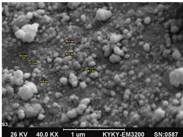
**Fig. 1** The scanning electron microscopy (SEM) image of  $\text{Fe}_3\text{O}_4\text{-BF}_3$  magnetic nanoparticles
