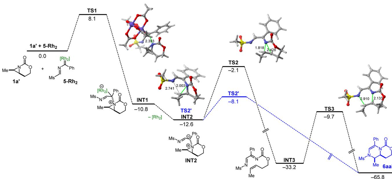
**Figure 2.** Computed reaction profile for the process involving **1a'** and dirhodium-bound carbene **5-Rh<sub>2</sub>**. Relative free energies ( $\Delta G$ , computed at 298.15 K and 1 M) and bond distances are given in kcal/mol and angstroms, respectively. All data have been computed at the SMD-B3LYP-D3/def2-SVP level.
