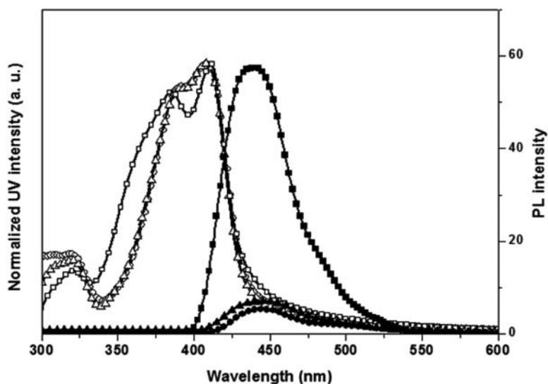
**Figure 2.** UV and PL spectrum of indenopyrazine derivatives in film on the glass ( $\bullet$  : DMP-EIP,  $\blacksquare$  : TFDMP-EIP,  $\blacktriangle$  : DPP-EIP).
