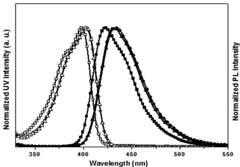
**Figure 1.** UV and PL spectrum of indenopyrazine derivatives in  $10^{-6}$  M  $\text{CHCl}_3$  solution ( $\bullet$  : DMP-EIP,  $\blacksquare$  : TFDMP-EIP,  $\blacktriangle$  : DPP-EIP).
