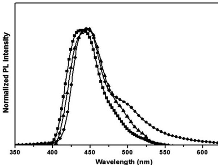
**Figure 3.** Normalized PL spectrum of indenopyrazine derivatives in film on the glass (● : DMP-EIP, ■ : TFDMP-EIP, ▲ : DPP-EIP).
