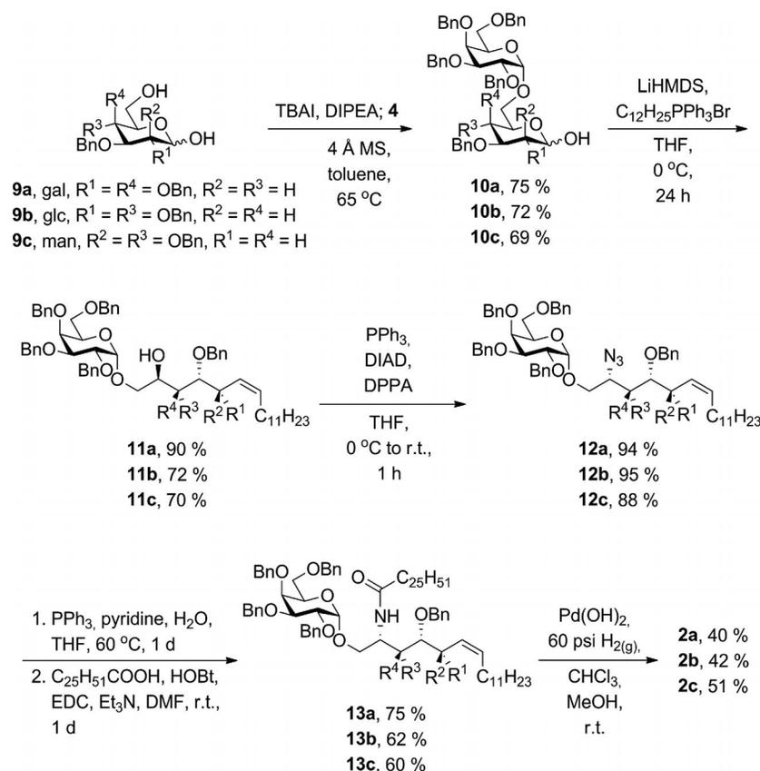
Scheme 1. Preparation of KRN7000 analogues **2a–2c**. DIAD = diisopropyl azodicarboxylate; DPPA = diphenylphosphoryl azide.
