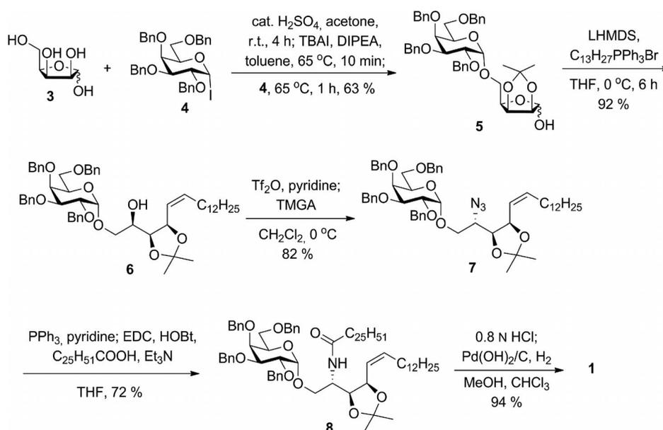
Figure 2. Previous report of the synthesis of KRN7000 in five steps.<sup>[8]</sup> TMGA = tetramethylguanidinium azide. EDC = 1-[3-(dimethylamino)propyl]-3-ethylcarbodiimide hydrochloride.
