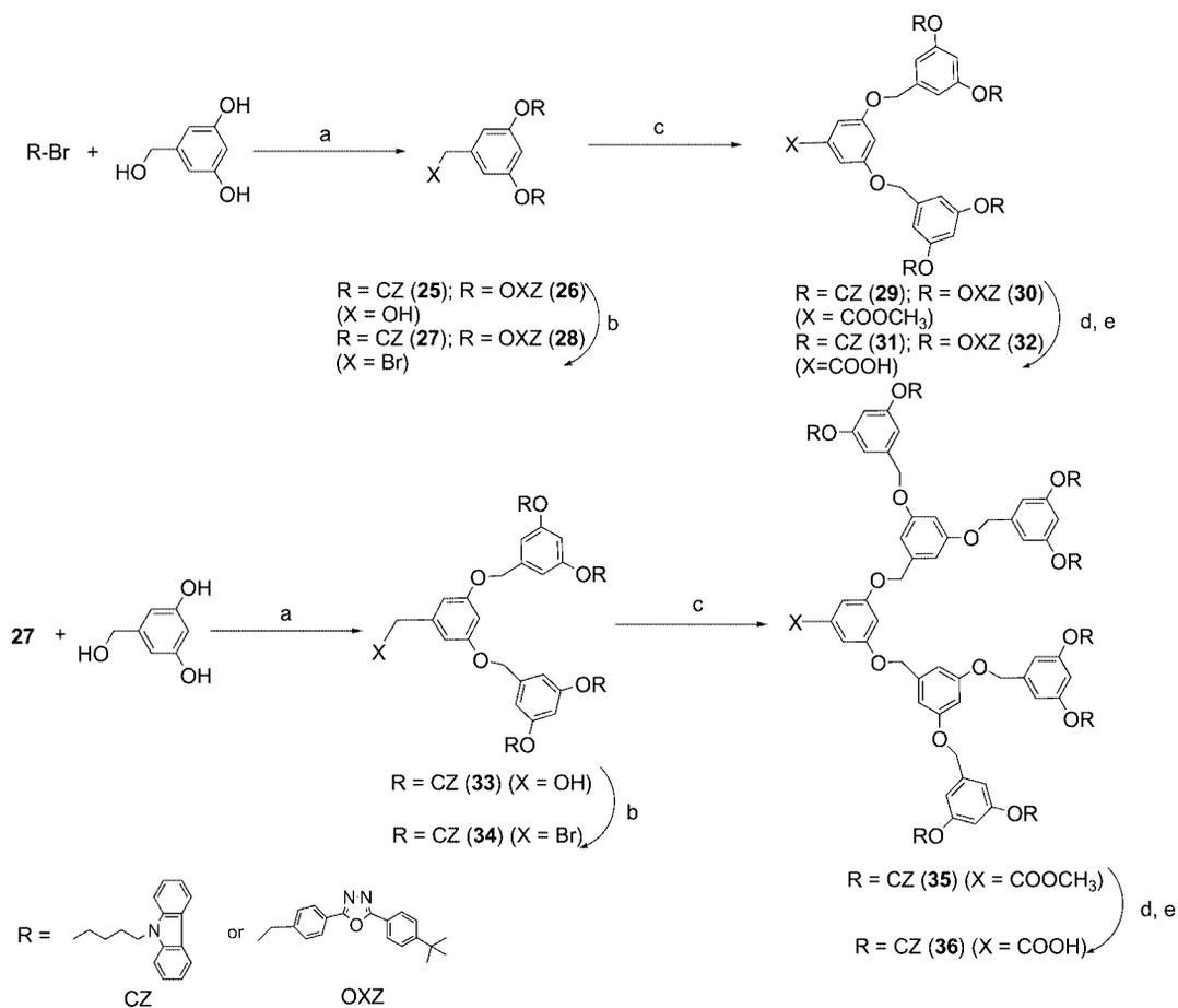
Scheme 5. Synthetic route to G-2 and G-3 dendrons of imide-type dendrimers. Reagents and conditions: a)  $K_2CO_3$ , 18-crown-6, acetone, reflux, 60 h; b)  $CBr_4/PPH_3$ ,  $CH_2Cl_2$ ; c) methyl 3,5-dihydroxybenzoate,  $K_2CO_3$ , 18-crown-6, THF, reflux, 60 h; d) KOH, THF/methanol, reflux; e) 10% HCl.
