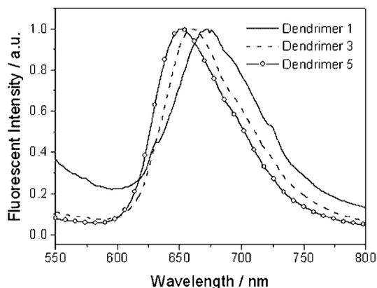
Figure 6. Normalized fluorescence spectra of dendrimers **1**, **3**, and **5** in solid film excited at 460 nm.
