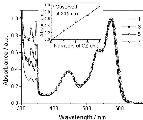
Figure 5. Normalized absorption spectra of dendrimers **1**, **3**, **5**, and **7** in THF ( $2.0 \times 10^{-5}$  M). Inset: Plot of number of carbazole units in dendrimer vs. absorbance at  $345$  nm.
