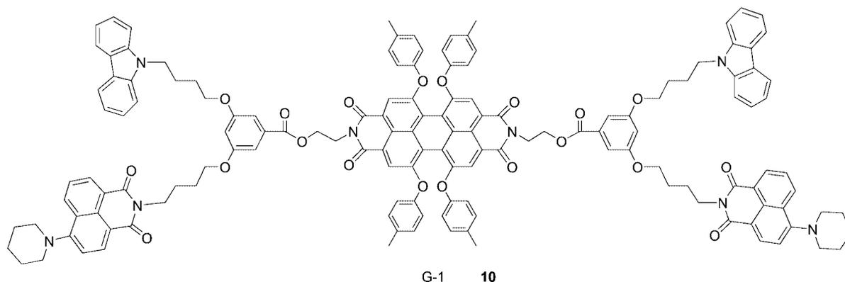
Scheme 2. Chemical structure of cascade energy-transfer imide-type dendrimers.
