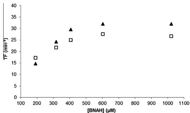
**Figure 3.** Turnover frequency (TF) with varying BNAH concentrations; P450<sub>Cl $\alpha$</sub>  (▲), P450<sub>Bs $\beta$</sub>  (□). Tris-HCl buffer (50 mM, pH 7.5), [myristic acid] = 200  $\mu$ M, [FMN] = 60  $\mu$ M, [P450] = 1  $\mu$ M (cell-free extracts), 30 °C, 5 min.
