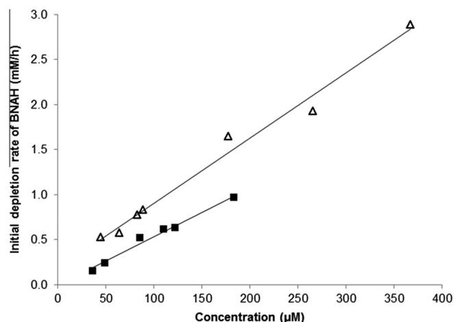
**Figure 1.** Initial depletion rate of BNAH with varying BNAH ( $\Delta$ ) concentration ([FMN] = 120  $\mu\text{M}$ ), and FMN ( $\blacksquare$ ) concentration ([BNAH] = 85  $\mu\text{M}$ ).
