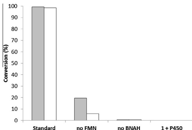
**Figure 5.** Product **2** and **3** formation with control reactions; P450<sub>C1α</sub> (grey), P450<sub>B5β</sub> (white). Tris-HCl buffer (50 mM, pH 7.5), [myristic acid] = 200 μM, [FMN] = 60 μM, [BNAH] = 600 μM, [P450] = 1 μM (purified enzyme), 30 °C, 20 min.
