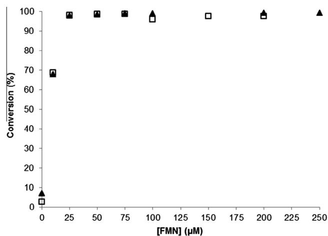
**Figure 4.** Product **2** and **3** formation with varying FMN concentrations; P450<sub>Cl $\alpha$</sub>  (▲), P450<sub>Bs $\beta$</sub>  (□). Tris-HCl buffer (50 mM, pH 7.5), [myristic acid] = 200  $\mu$ M, [BNAH] = 600  $\mu$ M, [P450] = 1  $\mu$ M (purified enzyme), 30 °C, 5 min.
