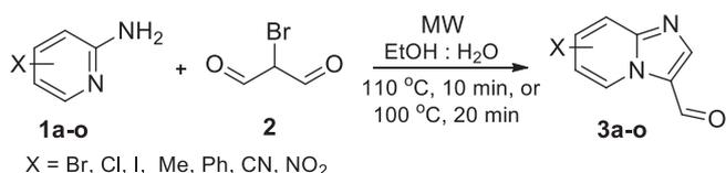
**Scheme 2.** Optimised conditions for the synthesis of imidazo[1,2-*a*]pyridine 3-carbaldehydes.
