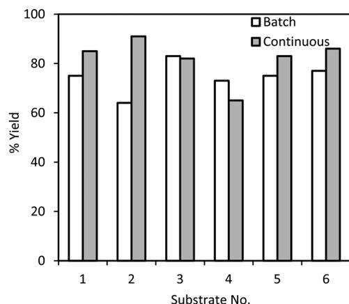
**Figure 3.** Comparison of yield from batch and continuous flow synthesis of various quinaldines for different anilines (1: aniline, 2: 3-nitroaniline, 3: *p*-toluidine, 4: *p*-anisidine, 5: *p*-chloroaniline, 6: 4-nitroaniline).
