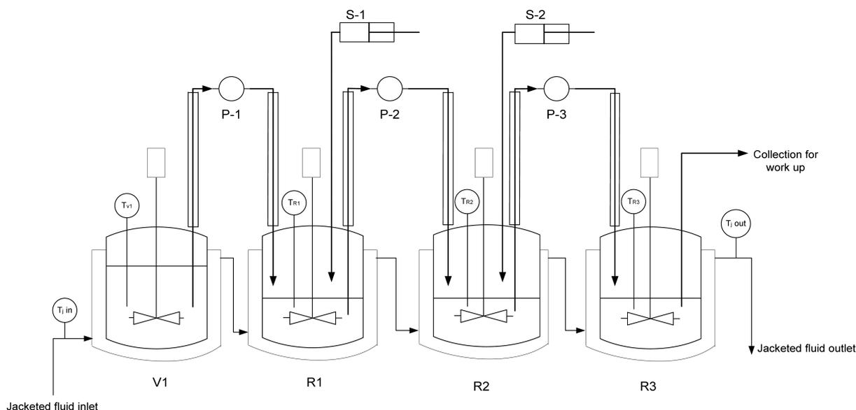
**Figure 1.** Schematic of continuous synthesis of quinaldine (P – pump, R – reactor, V – vessel, S – syringe pump, T – temperature indicators).
