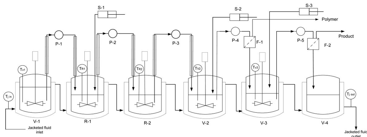
**Figure 2.** Schematic of continuous synthesis of quinaldine followed by continuous workup (P – pump, R – reactor, V – vessel, F – Filter, S – syringe pump [S1 – crotonaldehyde, S2/S3 – NaOH]).
