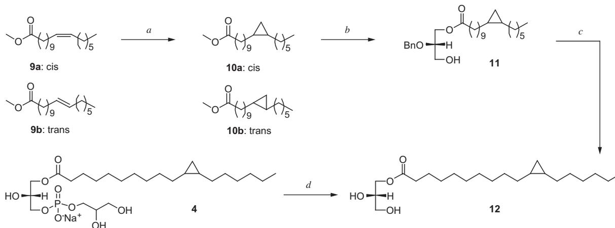
Scheme 2. Reagents and conditions: (a)  $\text{CH}_2\text{I}_2$ ,  $\text{Et}_2\text{Zn}$ , benzene,  $70\text{ }^\circ\text{C}$ , 6 h; (b) 2-*O*-benzylglycerol, lipase,  $\text{CHCl}_3$ ,  $30\text{ }^\circ\text{C}$ , 6 days; (c)  $\text{H}_2$ , Pd/C, MeOH, rt, 24 h; (d) phospholipase C, Tris-HCl buffer,  $\text{CaCl}_2$ , rt, 22 h.
