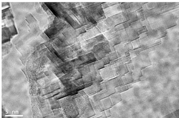
**Fig. 1** TEM image of nanocrystalline MgO**Table 2** Optimizing amount of nanocrystalline MgO and reaction temperature conditions on the formation of **2a**
