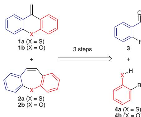
**Scheme 1** Retrosynthetic strategy for synthesizing six- and seven-membered oxygen- and sulfur-containing tricyclics from simple starting materials
