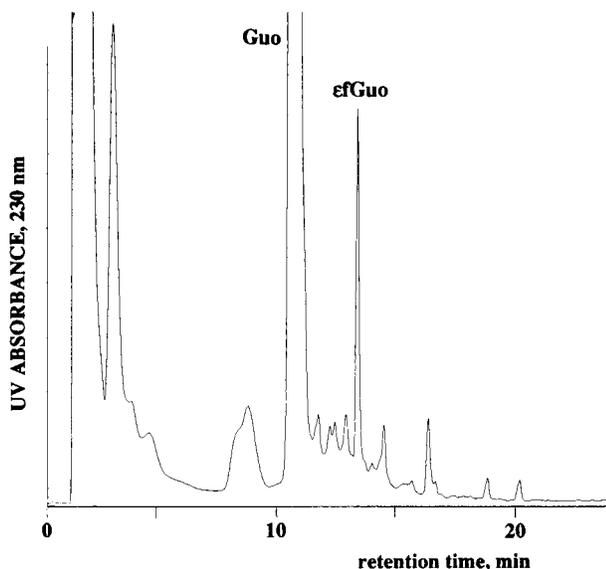
**Figure 1.** C18 column HPLC separation of the reaction mixture of MX and guanosine held at 37 °C and pH 8.2 for 6 days. For analysis conditions, see Materials and Methods.
