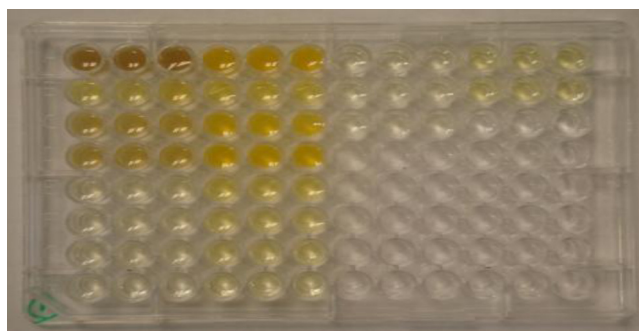
Fig. 1. Nessler's colorimetric activity assay towards 3-hydroxybutyronitrile, an example of library screening for nitrile-hydrolyzing enzyme activity in a 96-well plate format. The biotransformation was carried out at 25 °C with 10 mM nitrile. The reaction was then quenched by the addition of HCl. The biomass was removed by centrifugation. 20 \mu L of the supernatant was transferred to a microtitre plate, 181 \mu L of assay mastermix was added. The reaction was allowed to stand for 10 min and then the absorbance read at 425 nm.
