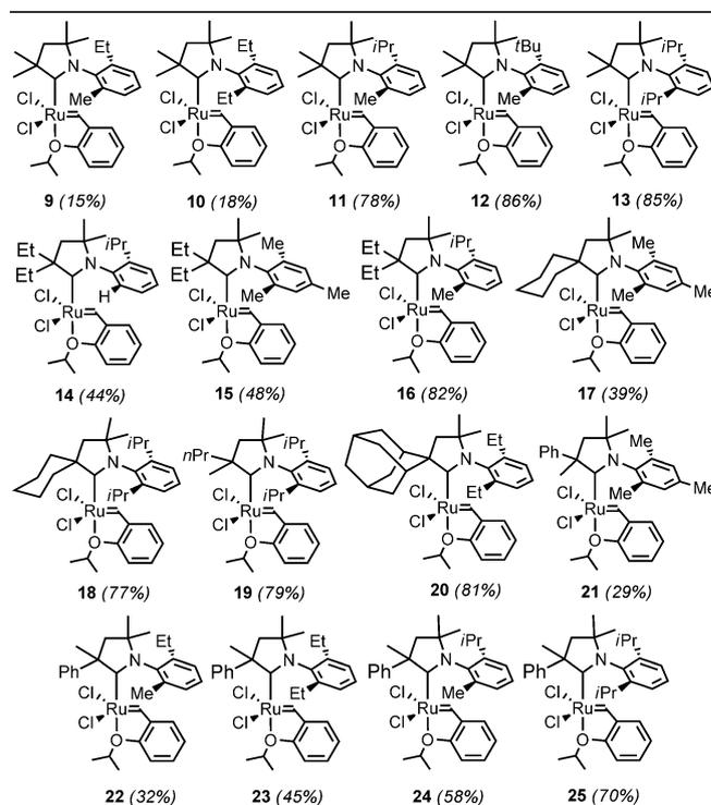
**Scheme 2.** Synthesis of the CAAC complexes under study (yields of isolated complexes in brackets).
