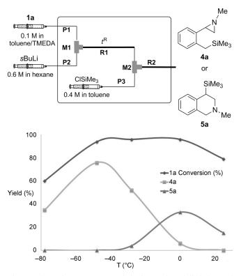
Figure 1. Flow microreactor for optimization of lateral lithiation and isomerization of **1a**. Reaction conditions:  $t^{R} = 23.56$  s; flow rates: aziridine 1a 3, sBuLi 1, electrophile 2 mLmin<sup>-1</sup>.<sup>[18]</sup>
