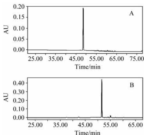
**Figure 7** The HPLC-UV chromatogram of mesaconitine (A) and 8-butyryl-benzoylmesaconine (B).
