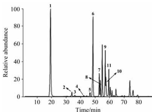
**Figure 3** HPLC chromatogram of metabolites of aconitine at pH 7. 1. benzoyleaconine, 2. 15-deoxybenzoyleaconine, 3. 8-octenoyl-benzoyleaconine, 4. 10-OH-aconitine, 5. 15-deoxyaconine, 6. aconitine, 7. 8-hexenoyl-benzoyleaconine, 8. 8-propionyl-benzoyleaconine, 9. 8-butyryl-benzoyleaconine, 10. deoxyaconitine, 11. 8(3-hydroxyl)-butyryl-benzoyleaconine.
