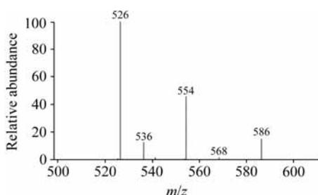
**Figure 4** The MS<sup>3</sup> spectrum of the 586 ion of peak 9.
