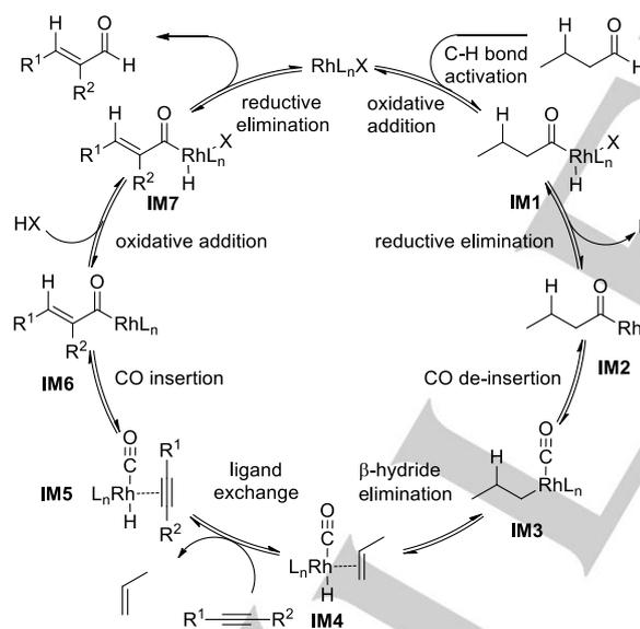
**Scheme 2.** Proposed mechanism involved in the transfer hydroformylation reaction of alkynes.
