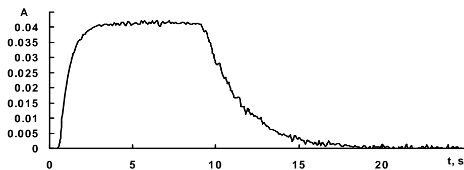
FIGURE S42. Kinetic curve for dibenzothienylethene 10 in toluene for processes of photocoloration under UV irradiation and photobleaching under visible light registered at 445 nm.
