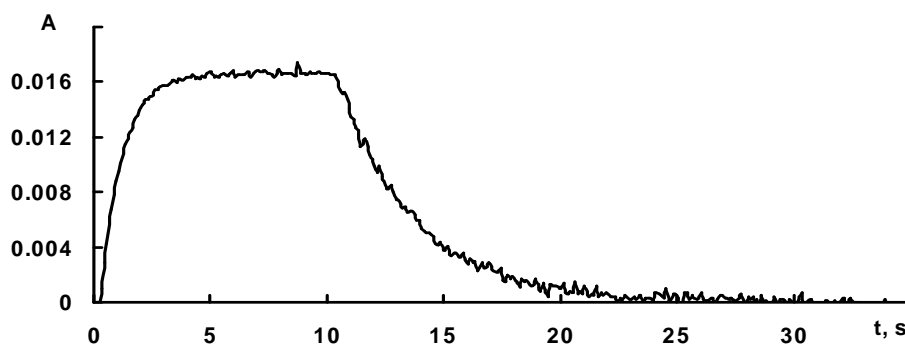
FIGURE S50. Kinetic curve for dibenzothienylethene 13 in acetonitrile for processes of photocoloration under UV irradiation and photobleaching under visible light registered at 445 nm.
