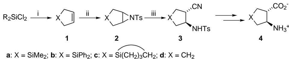
**Scheme 1.** Reagents and conditions: (i) Cp<sub>2</sub>TiCl<sub>2</sub> (5 mol%), H<sub>2</sub>C=CHMgBr (2.1 equiv.), THF, -40°C, 4 h; (ii) Chloramine-T (1.1 equiv.), PTAB (10 mol%), MeCN, rt, 5 h; (iii) Et<sub>2</sub>AlCN (4 equiv.), PhMe, 100°C, 17 h.
