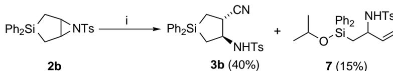
**Scheme 2.** Reagents and conditions: (i)  $\text{Me}_2\text{C}(\text{OH})\text{CN}$ ,  $\text{Yb}(\text{O}i\text{Pr})_3$ , THF,  $50^\circ\text{C}$ .
