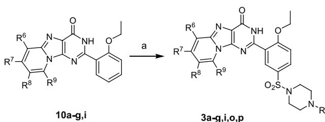
**Scheme 3.** Reagents and conditions: (a) (i) chlorosulfonic acid, 0–5 °C, 3 h; (ii) *N*-substituted piperazine, Et<sub>3</sub>N, CHCl<sub>3</sub>, rt, overnight.
