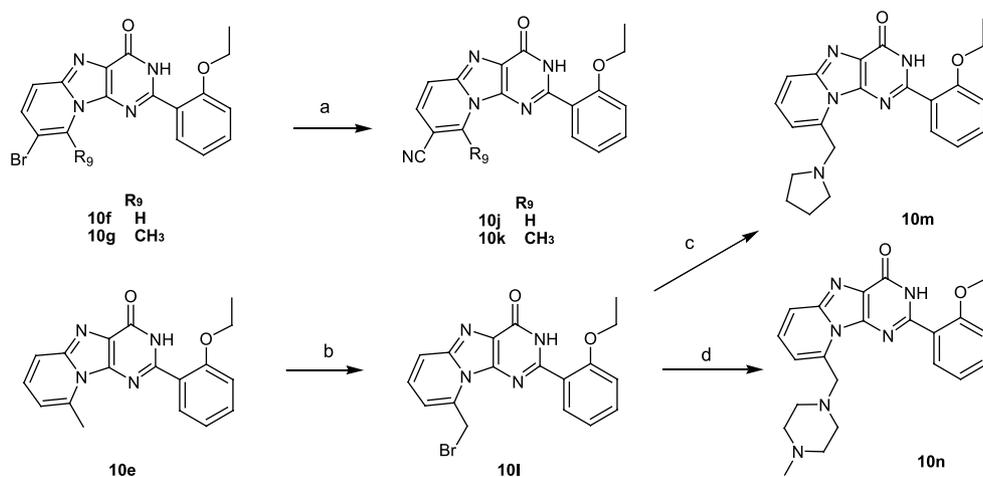
**Scheme 2.** Reagents and conditions: (a) NaCN, CuI, Pd(PPh<sub>3</sub>)<sub>4</sub>, DMF, reflux, 24 h; (b) NBS, CCl<sub>4</sub>, *hν*, 2 h; (c) pyrrolidine, K<sub>2</sub>CO<sub>3</sub>, acetone, rt, 20 h; (d) *N*-methylpiperazine, K<sub>2</sub>CO<sub>3</sub>, acetone, rt, 20 h.
