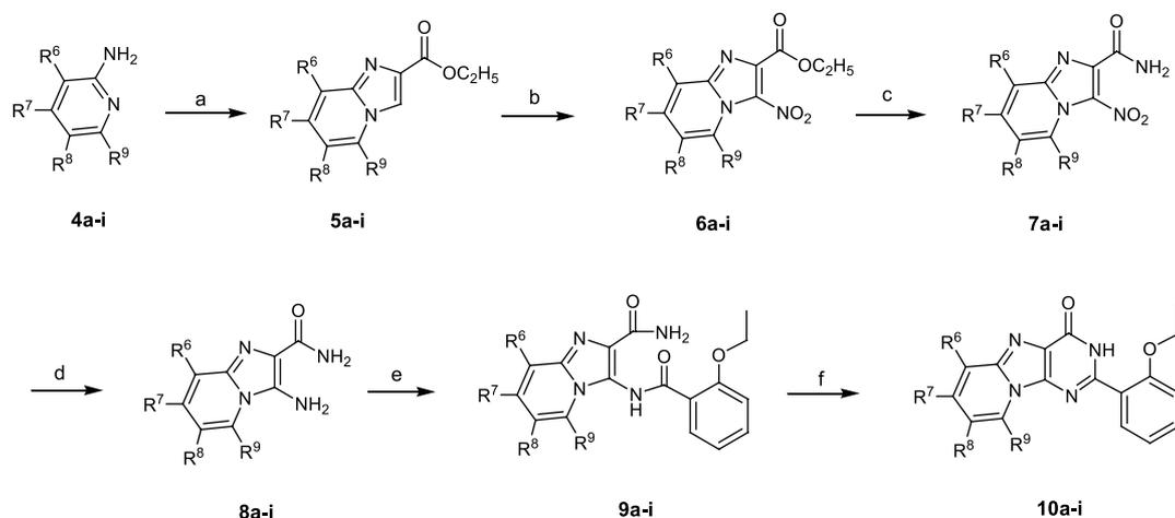
**Scheme 1.** Reagents and conditions: (a) ethyl bromopyruvate, EtOH, reflux, 6 h; (b) HNO<sub>3</sub>, H<sub>2</sub>SO<sub>4</sub>, –5–0 °C, 2 h; (c) NH<sub>4</sub>OH, H<sub>2</sub>O, THF, rt overnight; (d) H<sub>2</sub>, 10% Pt–C, 50 °C; (e) 2-ethoxybenzoyl chloride, pyridine, DMAP, CH<sub>2</sub>Cl<sub>2</sub>; (f) KO*t*-Bu, *t*-BuOH, reflux.
