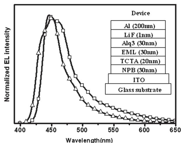
**Fig. 3.** EL spectra of OLED device using synthesized EML. The insert shows OLED device structure (DPP-EPY (-□-), DPBP-EPY (-Δ-)).
