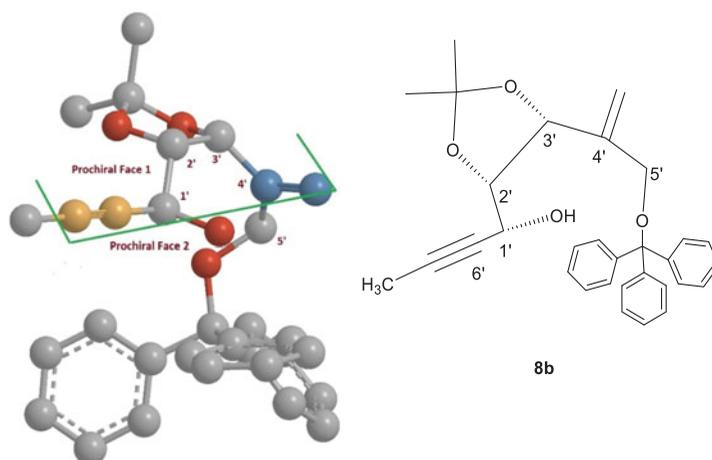
**Figure 2.** 3D structural pre-organization of **8b** before cyclization to show substrate controlled stereoselectivity. The Rh-catalyst system has approach only through prochiral face 1 using ligation with the acetonide followed by ligand exchange with the 1,6-ene-yne system. Prochiral face 2 is sterically crowded due to presence of trityl group.
