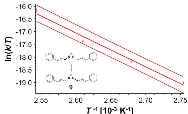
**Fig. 4.** Eyring plot of 1,2-dicinnamylidiaziridine **9** to determine the activation parameters of enantiomerization. The upper and lower curves represent the error bands of the linear regression with a level of confidence of 95%. For the linear regression, three measurements for each temperature were considered.
