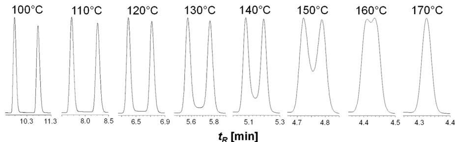
**Fig. 1.** Chromatograms of 1,2-diallyldiaziridine between 100 and 170°C. Separation conditions: 50 m × 250 μm i.d. fused-silica capillary coated with 250 nm heptakis(6-*O-tert*-butyldimethylsilyl)-2,3-di-*O*-ethyl)-β-cyclodextrin dissolved in polydimethylsiloxane PS086 (50% w/w), He as inert carrier gas.
