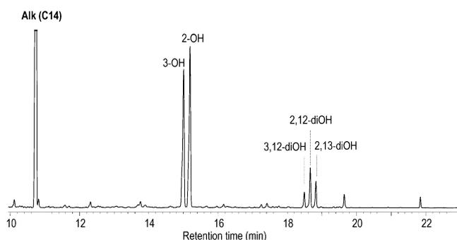
**Figure 1.** GC–MS analysis of the *AaeUPO* reaction with tetradecane, showing the remaining substrate (Alk, alkane) and the subterminal mono-/dihydroxylated (OH) derivatives (see the Supporting Information for details).
