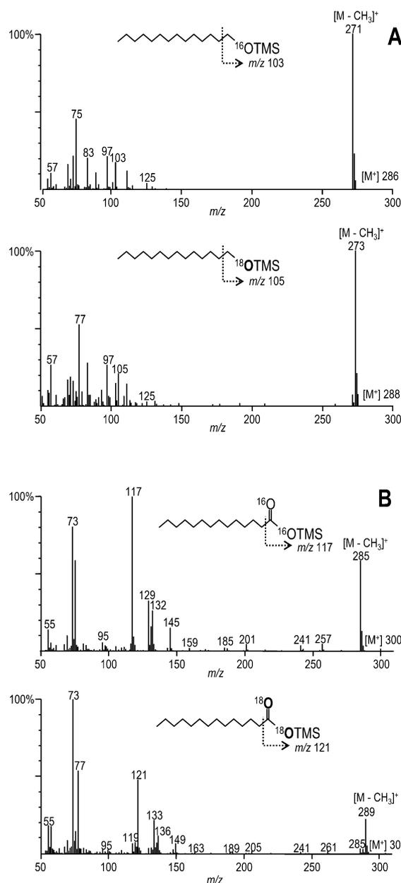
**Figure 4.** Mass spectra of 1-tetradecanol (A) and myristic acid (B) from *MroUPO* reactions with *n*-tetradecane in  $^{18}\text{O}$ -labeling experiments (bottom) and controls (top). The formulae for the unlabeled compounds found in the  $\text{H}_2^{16}\text{O}_2$  reactions (A and B, top) and the labeled compounds found in the  $\text{H}_2^{18}\text{O}_2$  (90% isotopic purity) reactions (A and B, bottom) are shown as trimethylsilyl (TMS) derivatives.
