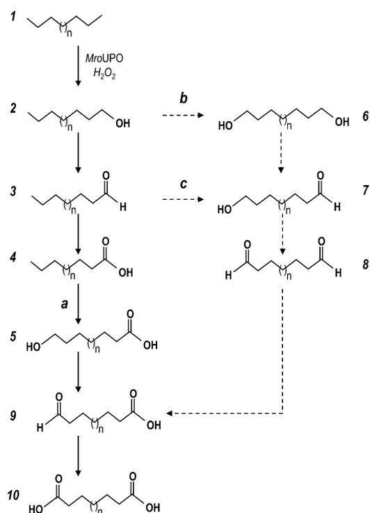
**Figure 3.** Pathways for the terminal oxygenation of *n*-alkanes to dicarboxylic acids, including identified and hypothetical intermediates, and three possible branch points (a, b and c) between mono- and dioxygenated compounds.
