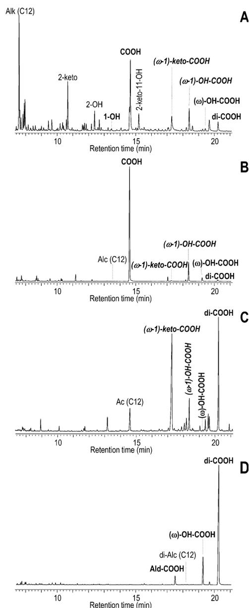
**Figure 2.** GC–MS analysis of *MroUPO* reactions with dodecane (A), 1-dodecanol (B), dodecanoic acid (C), and 1,12-dodecanediol (D) showing the remaining substrate (Alk, alkane; Alc, alcohol; and Ac, acid) and the terminal (bold), terminal/subterminal (bold, italics), and subterminal hydroxylated (OH) keto and carboxylic (COOH) derivatives (see the Supporting Information for details).
