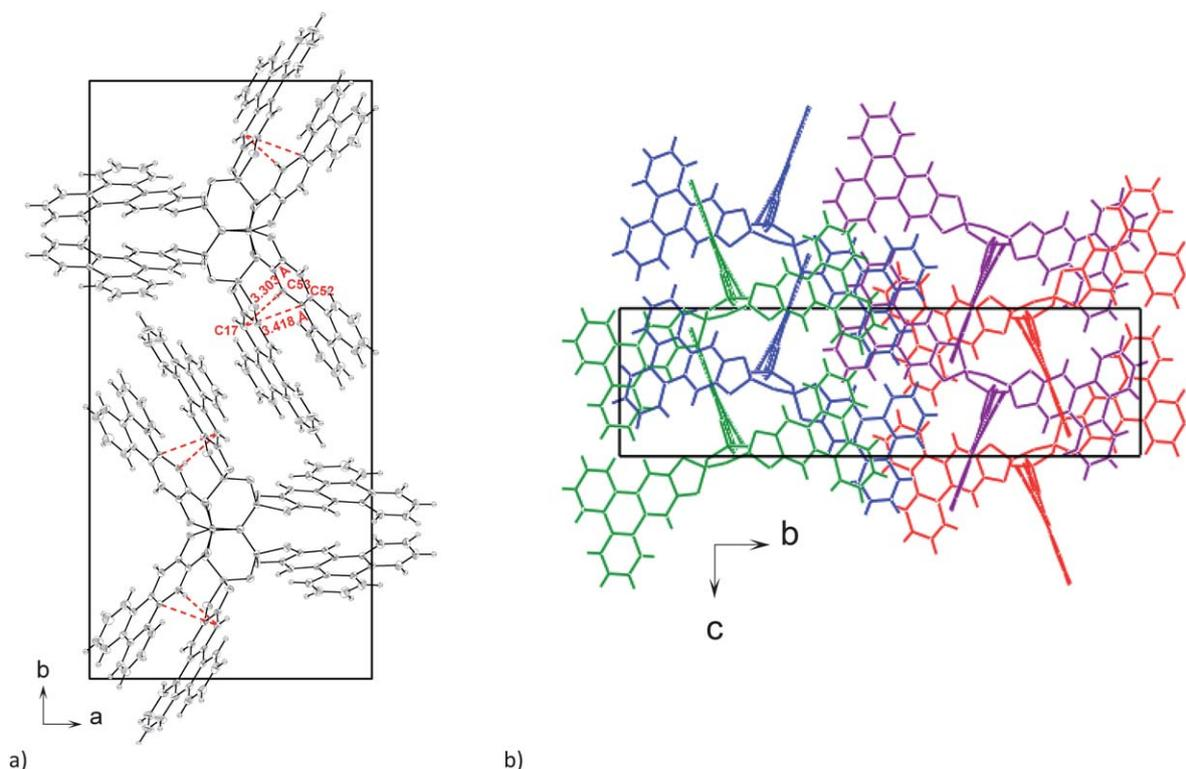
Fig. 2 TTPP in guest free crystal structure unit cell: a) View down  $c$ -axis ( $\pi$ – $\pi$  interactions between triphenylene units appear in red), b) View down  $a$ -axis. Molecules present a columnar arrangement along  $c$ -axis. Molecules are colored for clarity.
