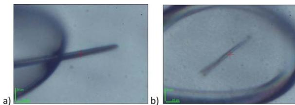
**Fig. 1** Photographs of a) TTPP **5** crystal and b) 1,2,4-trichlorobenzene–TTPP **5** inclusion adduct crystal on a nylon loop embedded with Paratone oil. The red cross indicates the beam position.
