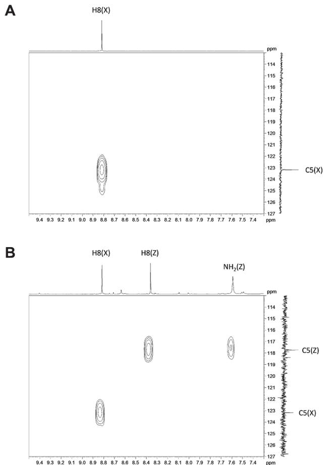
**Fig. 2** HMBC spectra of the modified nucleoside **1** (A) before and (B) after 5 h incubation in concentrated aq. ammonia at  $55\text{ }^\circ\text{C}$ , showing correlations between the C5 and H8 atoms of the purine ring and, in the case of the ammonolysis product, the hydrogen atoms of an exocyclic amino group. The spectra were measured in  $\text{DMSO-d}_6$ .
