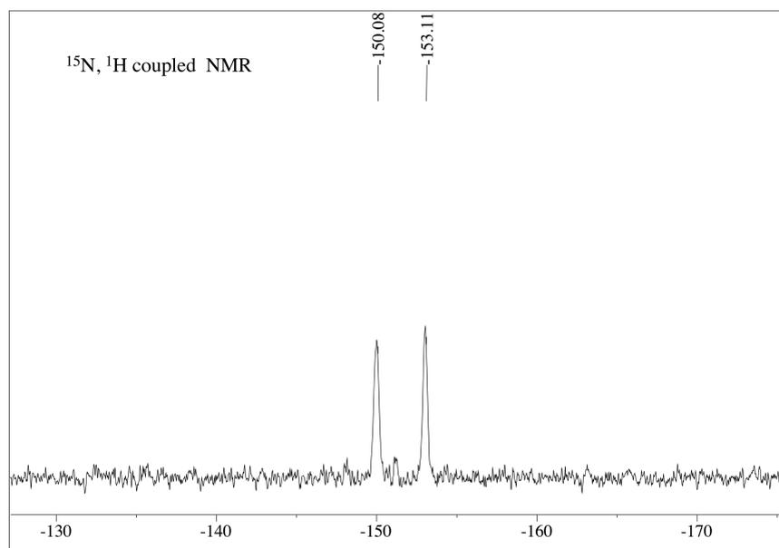
**Figure 6.**  $^{15}\text{N}$ ,  $^1\text{H}$  coupled NMR spectrum of  $[\text{Ru}(\eta^5\text{-C}_5\text{Me}_5)(\eta^2\text{-}^{15}\text{NH}=\text{NH})\{\text{P}(\text{OEt})_3\}_2]\text{BPh}_4$  (**71**) in  $\text{CD}_2\text{Cl}_2$  at 243 K.
