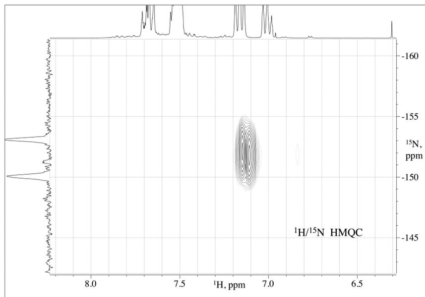
**Figure 5.** <sup>1</sup>H/<sup>15</sup>N HMQC NMR spectrum of [Ru( $\eta^5$ -C<sub>5</sub>Me<sub>5</sub>)( $\eta^2$ -<sup>15</sup>NH=NH){P(OEt)<sub>3</sub>}<sub>2</sub>]BPh<sub>4</sub> (**7**<sub>1</sub>) in CD<sub>2</sub>Cl<sub>2</sub> at 243 K.
