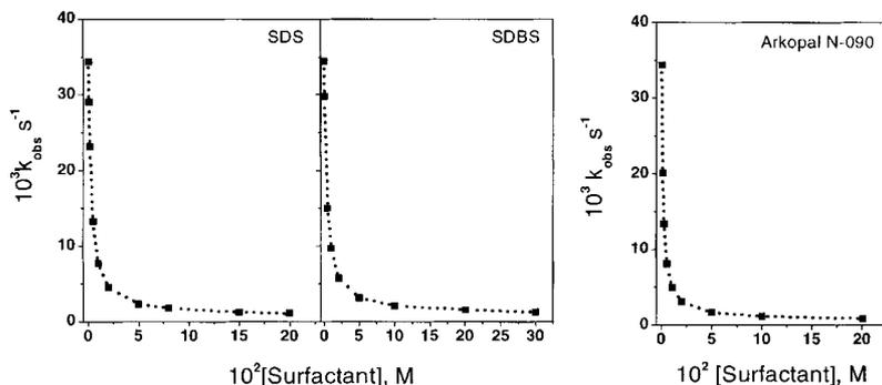
**Figure 1.** Dependence of observed rate constants,  $k_{\text{obs}}$ , on [surfactant] for anionic and non-ionic micelles at 35 °C. The points are experimental and the curves were calculated using Eqn. (1)
