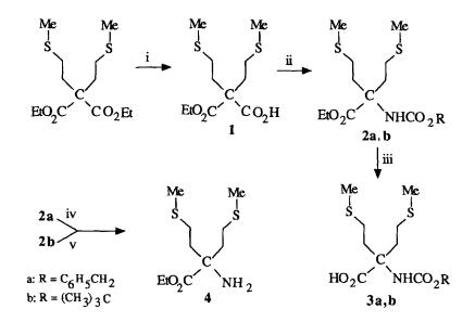
Reagents: i) KOH/dry EtOH; ii) DPPA, TEA, ROH; iii) NaOH/aqueous MeOH; iv) HCO<sub>2</sub>NH<sub>4</sub>, Pd/C; v) CF<sub>3</sub>CO<sub>2</sub>H/CHCl<sub>3</sub>
