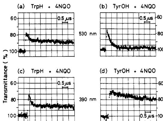
**Figure 2.** Oscilloscope traces of the changes in transmission at 530 (a, b) and 390 nm (c, d) observed for solutions 1 and 2 which are noted in the legend of Figure 1.
