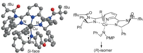
**Figure 3.** Proposed transition state for the alkynylation of an imine by using **1f**–Cu<sup>I</sup>.
