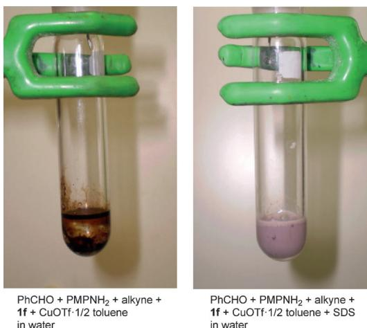
Figure 1. Homogenized reaction mixture after the addition of SDS.
