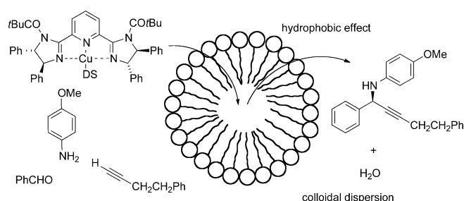
**Figure 2.** Three-component reaction in water by using a hydrophobic chiral catalyst.
