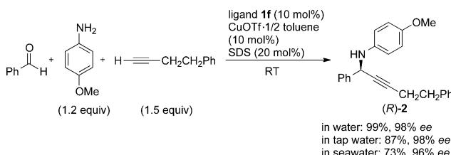
Scheme 1. Enantioselective three-component reaction in tap water and seawater.
