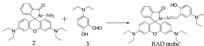
**Scheme 1.** Synthesis and the structure of RAD probe
