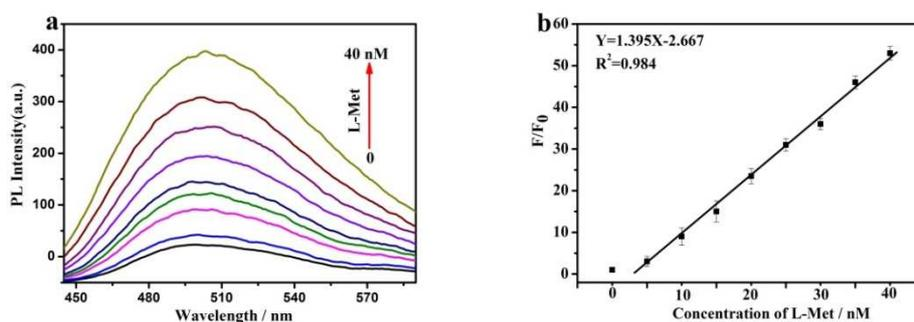
**Fig.3** (a) Fluorescence response of RAD-Cu<sup>2+</sup> system in the presence of increasing concentration of L-Met (from up to down the concentration of L-Met is 0, 5, 10, 15, 20, 25, 30, 35 and 40 nM). (b) The linear relationship of  $F/F_0$  versus the concentration of L-Met over the range from 0 to 40 nM ( $\lambda_{ex}=400$  nm).
