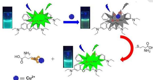
**Scheme 2** Mechanism of the “off-on” detection of  $\text{Cu}^{2+}$  and L-Met.
