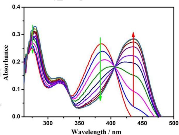
**Fig. 1** UV-vis titration spectra of RAD (10 µM) upon the gradual addition of Cu<sup>2+</sup> (0-40 nM).
