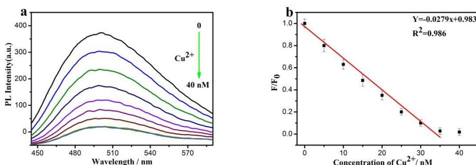
**Fig.2** (a) Fluorescence response of RAD in the presence of increasing concentration of  $\text{Cu}^{2+}$  (from up to down the concentration of  $\text{Cu}^{2+}$  is 0, 5, 10, 15, 20, 25, 30, 35 and 40 nM). (b) The linear relationship of  $F/F_0$  versus the concentration of  $\text{Cu}^{2+}$  over the range from 0 to 40 nM.  $\lambda_{\text{ex}}=400$  nm.
