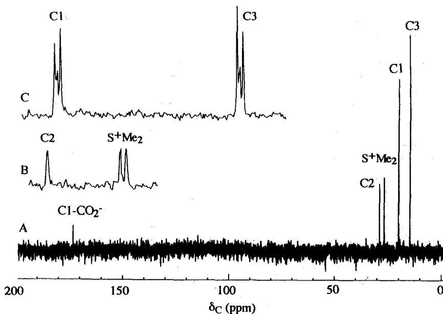
Fig. 1. 67.5 MHz Proton-decoupled  $^{13}\text{C}$  NMR spectrum of gonyauline in  $\text{D}_2\text{O}$  isolated from *Gonyaulax polyedra* cultured in the presence of [2,3- $^{13}\text{C}_2$ ]methionine (entry 3): (A) all carbons; (B) expansion of C2 and  $\text{S}^+\text{Me}_2$ ; and (C) expansion of C1 and C3.
