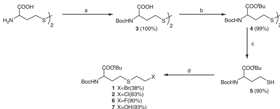
**Scheme 1.** Synthesis of precursors 1-2. Reagents and conditions: (a)  $\text{Boc}_2\text{O}$ , dioxane,  $\text{Na}_2\text{CO}_3(\text{aq})$ , RT; (b) *tert*-butyl-2,2,2-trichloroacetimidate,  $\text{CH}_2\text{Cl}_2$ , RT; tributylphosphine, DMF, RT; and (d) 1-bromo-2-haloethane or 2-bromoethanol,  $\text{K}_2\text{CO}_3$ , DMF, RT.2
