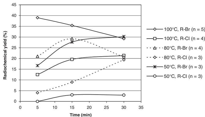
**Figure 1.** Radiolabelling of bromo- and chloro-precursors **1** and **2** (5 mg) in acetonitrile (1 mL) with  $K_{222}$  (10 mg) and  $K_2CO_3$  (2 mg) as a function of temperature and time.
