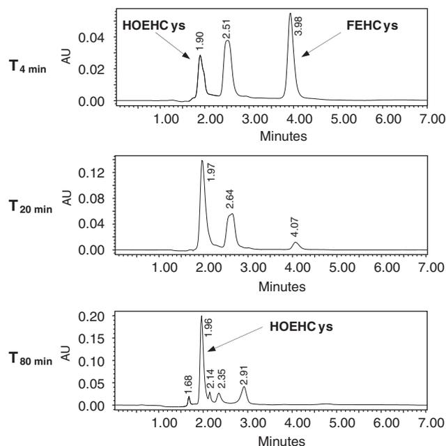
**Figure 2.** Investigation of the stability of FEHCys by HPLC (sample: 1 mg of a 95:05 mixture of FEHCys and HOEHCys in 500  $\mu$ L of water; HPLC conditions: Grace AlltimaC18 column (150  $\times$  4.6 mm, 5  $\mu$ m); mobile phase  $CH_3CN/H_2O$  10/90, v/v; flow rate 1 mL/min;  $\lambda$  = 210 nm).
