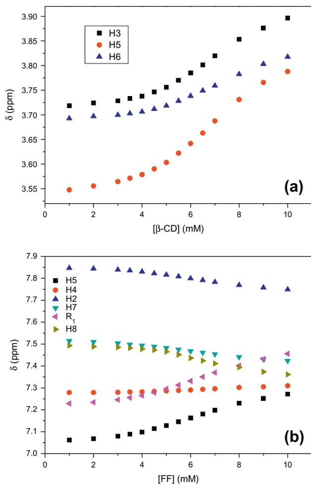
**Fig. 5.** Chemical shifts variation of some representative: (a)  $\beta$ -CD and (b) FF protons as a function of their concentration, ( $[\beta\text{-CD}] + [\text{FF}] = 10 \text{ mM}$ ).
