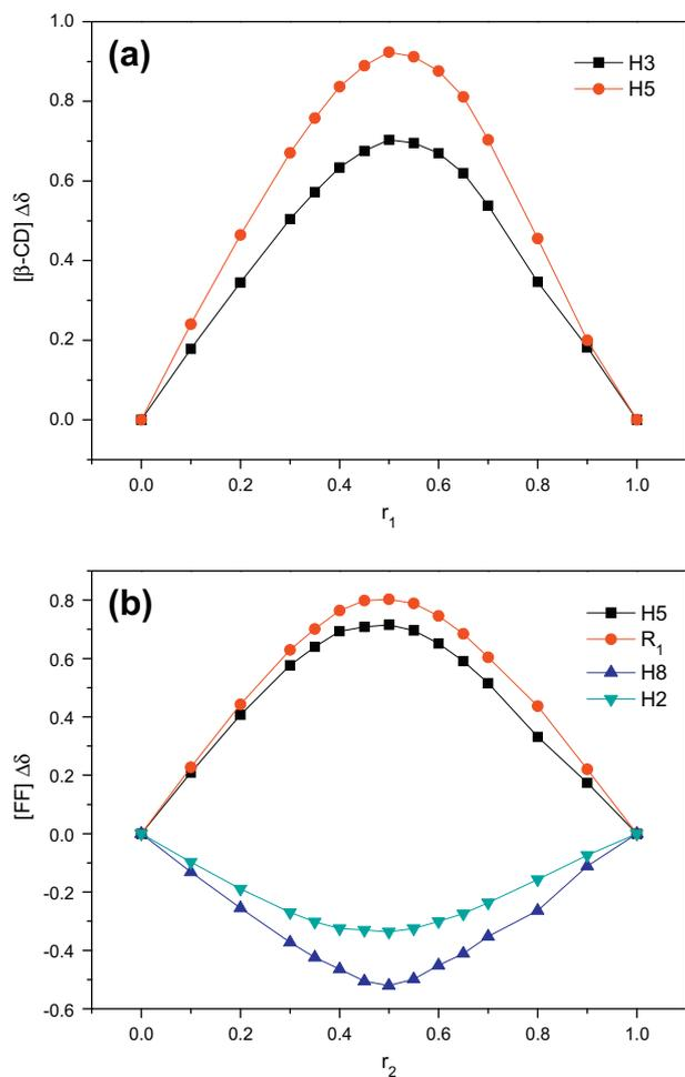
Fig. 7. Job's plots corresponding to the induced chemical shift variation of some: (a)  $\beta$ -CD and (b) FF protons for the FF:  $\beta$ -CD system.
