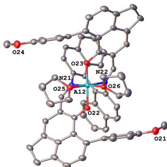
**Figure 1.** X-ray crystal structure of *rac*-9-BPh<sub>4</sub>, depicting the restricted catalyst binding pocket. Only one of the two independent molecules is shown; counterions, solvent, and H atoms are omitted for clarity. Displacement ellipsoids shown at 50% probability.
