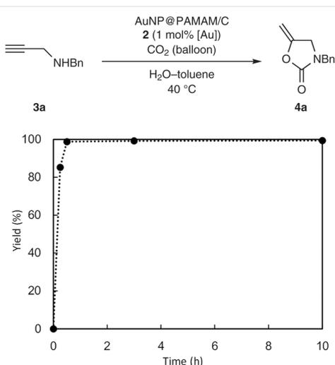
**Figure 2** Time-course curve of the carboxylative cyclization of a propargylic amine **3a**
