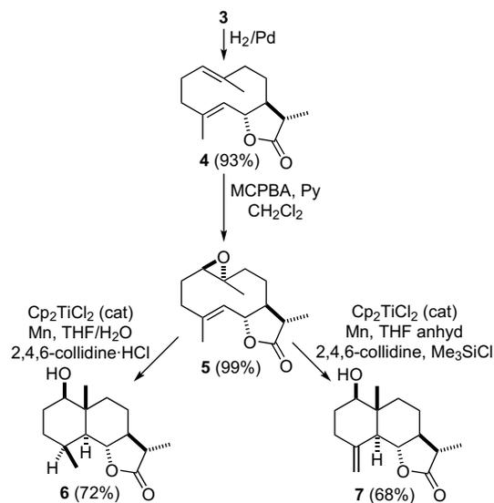
**Scheme 3.**  $\text{Ti}^{\text{III}}$ -catalyzed synthesis of intermediates **6** and **7**.
