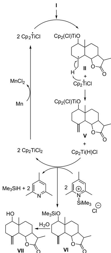
**Scheme 4.** Hypothetical catalytic cycle for  $\text{Ti}^{\text{III}}$ -catalyzed transannular cyclization of 1,10-epoxygermacrolides under anhydrous conditions.
