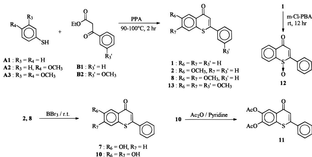
PPA: polyphosphoric acid; m-Cl-PBA: m-Chloro benzoic acid peroxide.
