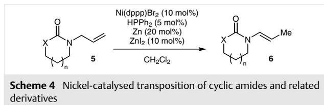
**Scheme 4** Nickel-catalysed transposition of cyclic amides and related derivatives
