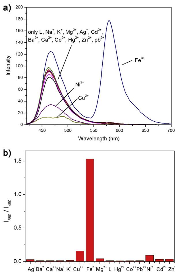
**Fig. 3.** a) The fluorescence spectra of 10  $\mu\text{M}$  **L** in buffered EtOH/HEPES = 99:1 solution at pH 7.2 with 5 equiv. metal ions:  $\text{Ba}^{2+}$ ,  $\text{Ca}^{2+}$ ,  $\text{Cd}^{2+}$ ,  $\text{Co}^{2+}$ ,  $\text{K}^+$ ,  $\text{Mg}^{2+}$ ,  $\text{Na}^+$ ,  $\text{Ag}^+$ ,  $\text{Fe}^{3+}$ ,  $\text{Pb}^{2+}$ ,  $\text{Hg}^{2+}$ ,  $\text{Ni}^{2+}$ ,  $\text{Cu}^{2+}$  ions and blank. b) The ratio of fluorescence intensity (580 nm/460 nm) of **L** and **L** with metal ions.
