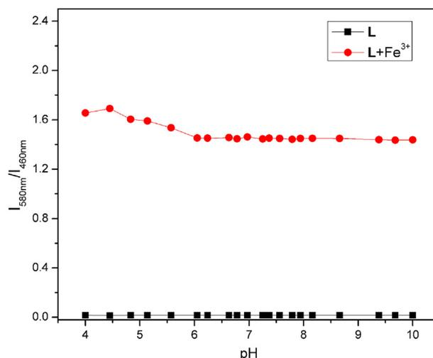
**Fig. 4.** The effect of pH (4.0–10.0) on the fluorescence intensity ratio (580 nm/460 nm) of 10  $\mu\text{M}$  probe **L** with 5.0 equiv.  $\text{Fe}^{3+}$  in buffered EtOH/HEPES solution.
