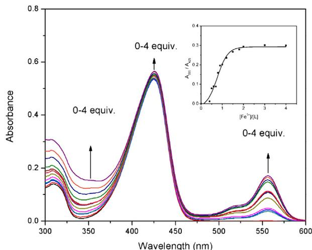
Fig. 1. Absorption spectra of 10  $\mu\text{M}$  **L** upon the addition of  $\text{Fe}^{3+}$  (0–4 equiv.) in buffered EtOH/HEPES = 99:1 solution at pH 7.2. The inset shows the ratio of the absorbance (555 nm/425 nm) as a function of  $\text{Fe}^{3+}$  concentration.
