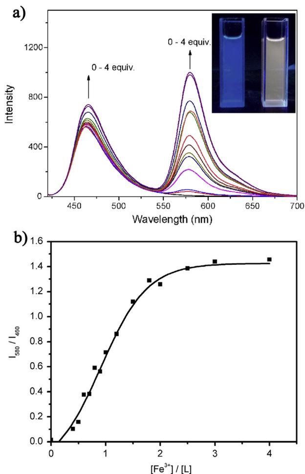
**Fig. 2.** a) The fluorescence spectra of 10  $\mu$ M **L** upon the addition of 0–4 equiv  $Fe^{3+}$  in buffered EtOH/HEPES = 99:1 solution at pH 7.2. The inset shows the fluorescence photo of **L** and **L-Fe<sup>3+</sup>**. b) The ratio of fluorescence intensity (580 nm/460 nm) of **L** as a function of  $Fe^{3+}$  concentration.
