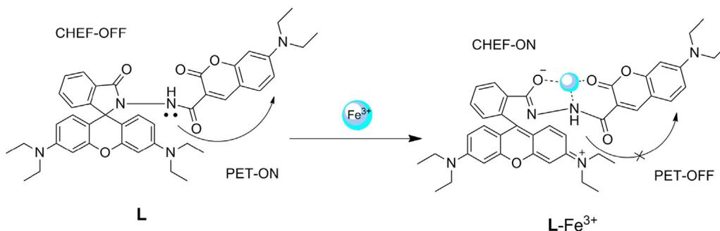
**Scheme 2.** Proposed complex mechanism of **L-Fe<sup>3+</sup>**.
