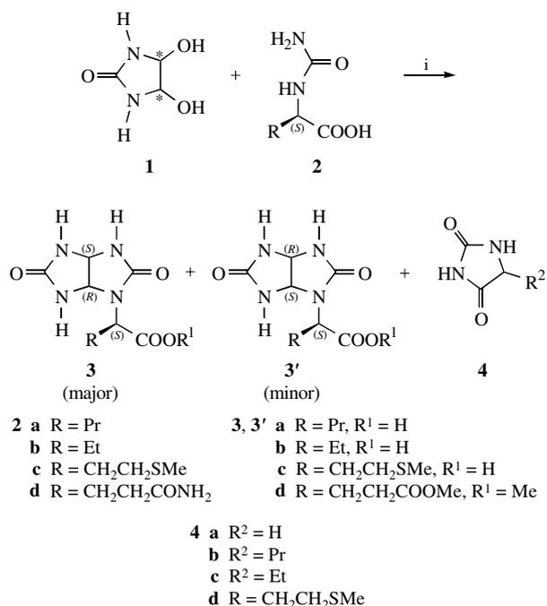
**Scheme 1** Reagents and conditions: i, H<sub>2</sub>O (H<sub>2</sub>O/Pr<sup>i</sup>OH), HCl, 90 °C, 1 h.
