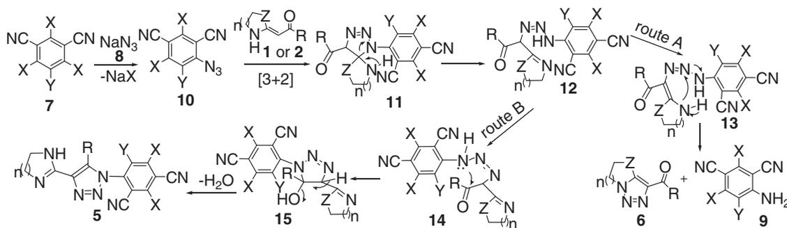
**Scheme 3.** Proposed mechanism for the formation of 1,2,3-triazoles.
