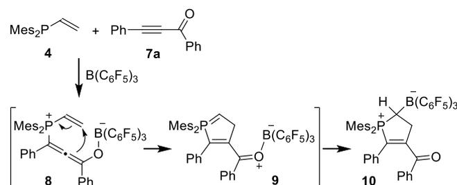
Scheme 2. Formal enphosphane plus ynone [3+2] cycloaddition in the presence of stoichiometric  $B(C_6F_5)_3$ .
