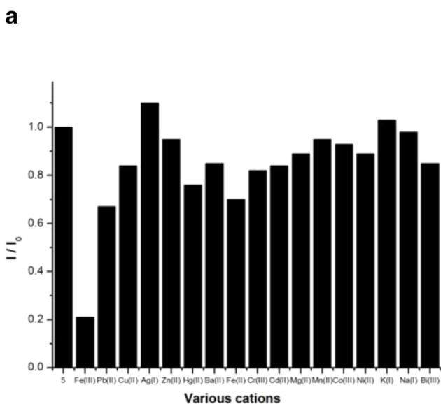
**Fig 2 a** Relative fluorescence intensity changes of QQ in the presence of various metal ions(10 eq.) in HEPES buffer solution (10 mM, pH=7.0, DMF-H<sub>2</sub>O, 9:1, v/v), λ<sub>ex</sub>=344 nm. **b** Fluorescence spectra of QQ in the
