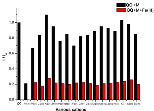
**Fig 3** Relative fluorescence intensity changes of QQ in the presence of various metal ions (20 eq.) and Fe<sup>3+</sup> (20 eq.) in HEPES buffer solution (10 mM, pH=7.0, DMF-H<sub>2</sub>O, 9:1, v/v).λ<sub>ex</sub>=344 nm
