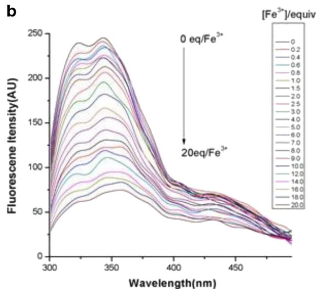
presence of various equiv of Fe<sup>3+</sup> in HEPES buffer solution (10 mM, pH=7.0, DMF-H<sub>2</sub>O, 9:1, v/v).λ<sub>ex</sub>=344 nm
