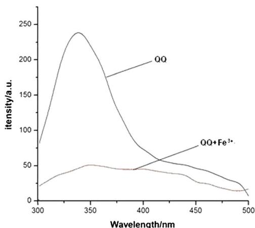
**Fig 1** Fluorescence emission spectra of QQ in the presence of Fe<sup>3+</sup> in HEPES buffer solution (10 mM, pH=7.0, DMF-H<sub>2</sub>O, 9:1, v/v), λ<sub>ex</sub>=344 nm
