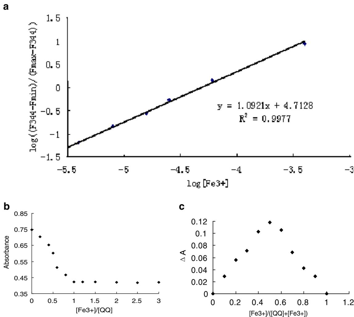
**Fig 4** **a** Curve of fluorescence intensity at 344 nm of QQ versus increasing concentration of  $\text{Fe}^{3+}$ . **b** Absorbance of QQ- $\text{Fe}^{3+}$  complex in different  $[\text{Fe}^{3+}]/[\text{QQ}]$  ratio. **c** Job's plot for the QQ- $\text{Fe}^{3+}$  complex ( $[\text{QQ}] + [\text{Fe}^{3+}] = 5 \times 10^{-5} \text{ mol dm}^{-3}$ )
