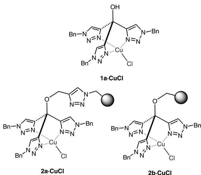
**Figure 2.** Homogeneous (**1a**·CuCl) and heterogenized (**2a**·CuCl and **2b**·CuCl) catalysts for CuAAC with the tris(triazolyl)methanol (TTM) structure.
