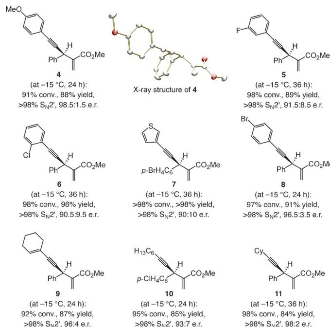
**Scheme 2.** A range of products can be accessed in high efficiency and site- and enantioselectivity through catalytic EAS. Reactions were performed under the conditions shown in Table 1 (**1a** as catalyst precursor); 0.5 mol % **1a** and 1.0 mol % Cu salt used for EAS affording **7** and **11**.
