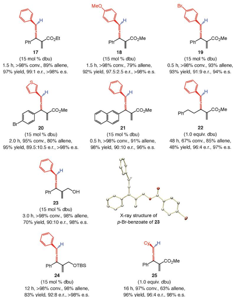
**Scheme 5.** Trisubstituted allenes can be accessed efficiently in high enantiomeric purity through dbu-catalyzed isomerization; the X-ray structure of a derivative of **23** supports the *syn* mode of proton transfer. Yields correspond to mixtures of isomers.
