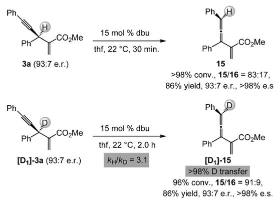
**Scheme 4.** Alkyne-to-allene isomerization proceeds to completion within 30 min; labeling experiment indicates a significant primary kinetic isotope effect. Yields correspond to mixtures of isomers; see the Supporting Information for details.
