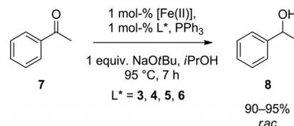
Scheme 7. Conditions for catalytic hydrogen transfer from literature.<sup>[18]</sup> Neither  $\text{Fe}^{\text{II}}$ ,  $\text{L}^*$ , or triphenylphosphane are necessary to obtain the conversions reported.
