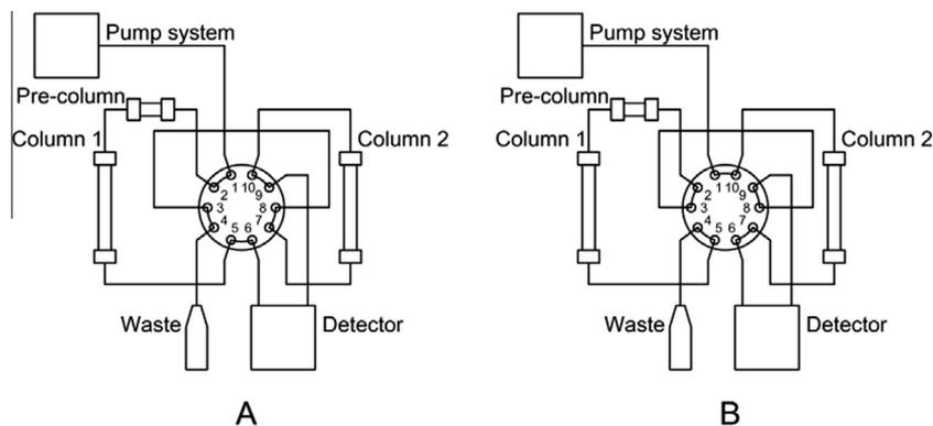
Fig. 2. Principle of the sample recycle HPLC equipment. The two different figures correspond to the both positions of the valve. (A) col. 1 → UV → col. 2, (B) col. 2 → UV → col. 1.
